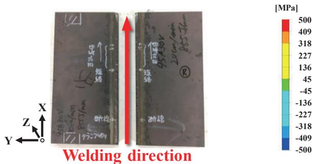
Fig. 17 Bead on plate welding Specimen.
