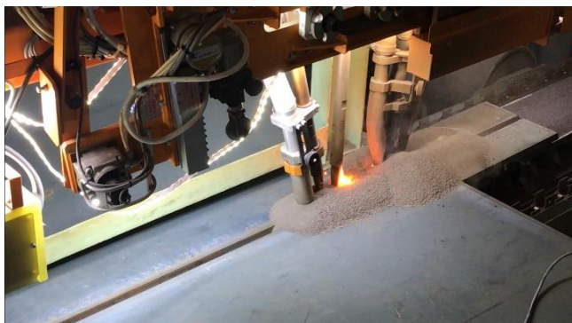
Fig. 1 Photo of Multiple Electrode Single-sided Submerged Arc Welding.
