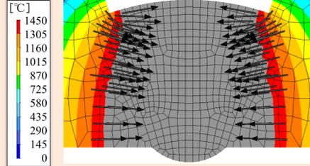
BTR Temperature Gradient Vector : Temperature gradient in the BTR during cooling
