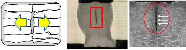
Hot cracking may decrease the strength of the structure. Repair welding necessary if it is occurred.
