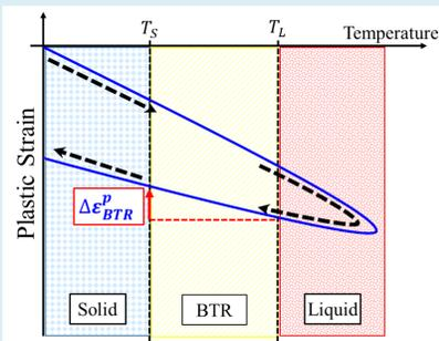
BTR plastic strain increment: Plastic strain increment  $\Delta\varepsilon^p$  in the BTR during cooling
