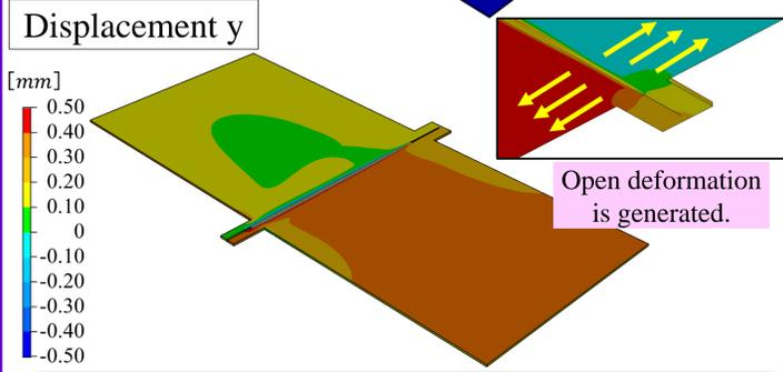
Sequential analysis with moving heat source is performed.
