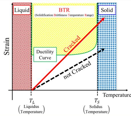
Evaluation of strain on weld metal during BTR by FEM analysis.
