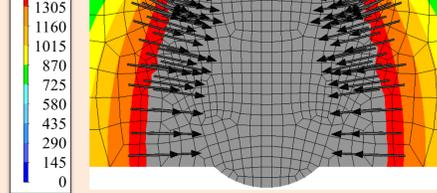
BTR Temperature Gradient Vector : Temperature gradient in the BTR during cooling
