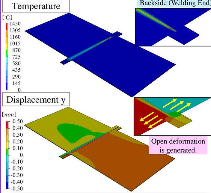
Sequential analysis with moving heat source is performed.
