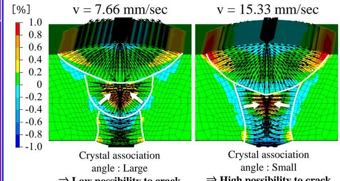
Small welding speeds may reduce hot cracking.
