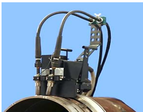
Fig. 1 Tandem torches used in pipe welding.
