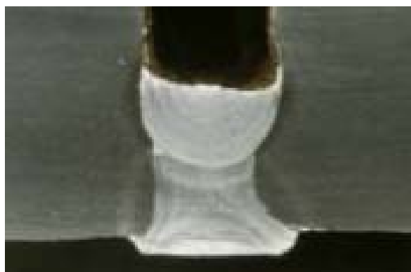
Fig. 9 Photo of penetrated shape of 2 torch MAG welding.
