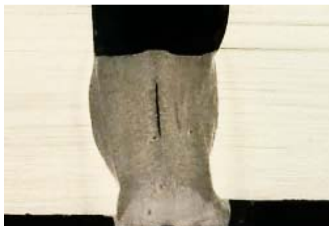
Fig. 2 Photo of solidification cracking under high-speed narrow gap welding with tandem torches.
