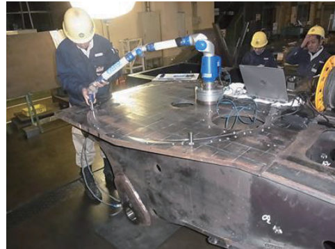
Fig. 7 Photograph of measurement using FARO.
