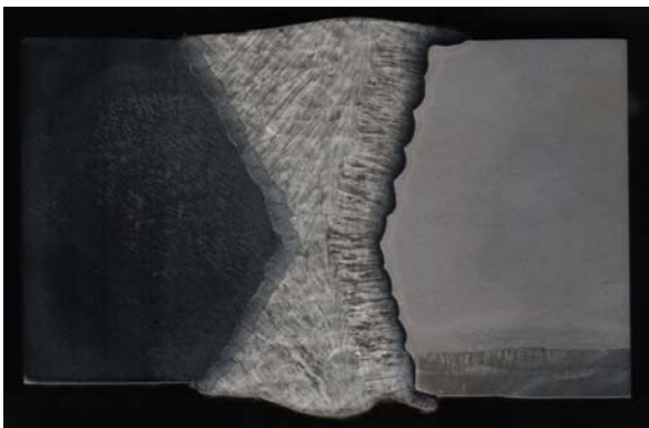
Fig. 7 Cross section of weld joint.
