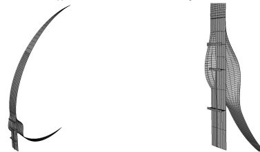
Fig. 6 Initial deflection shape of analyzed sphere tank
